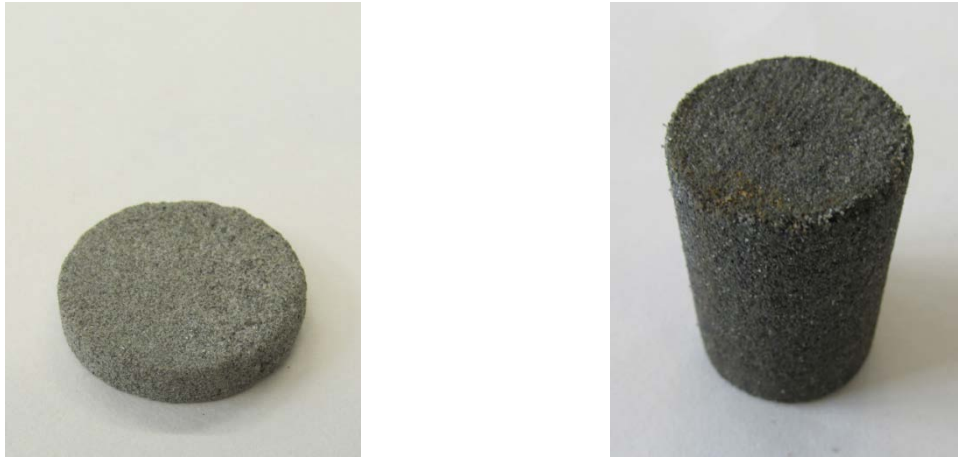
Figure 35: Photos of the cores from the NU original sample (left) and after storage (right)
