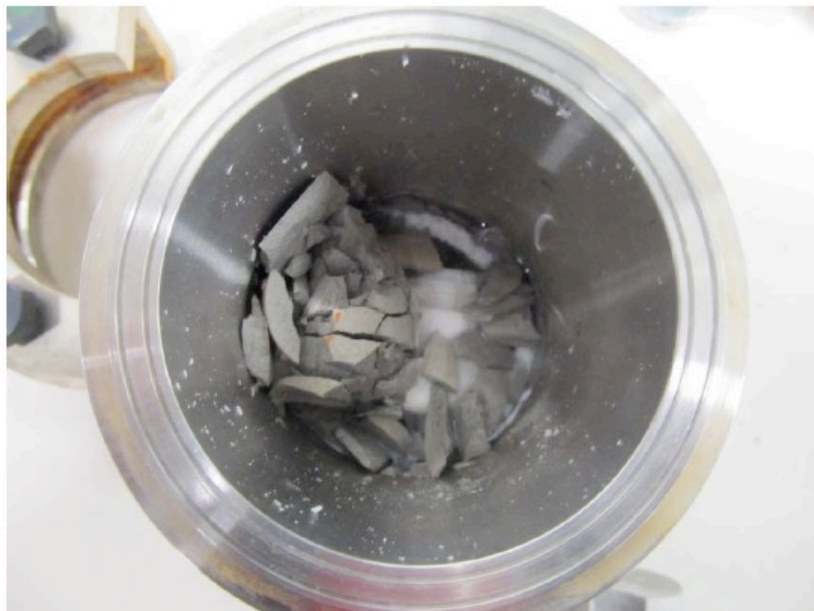
Figure 82: Fragmented core after autoclave opening
