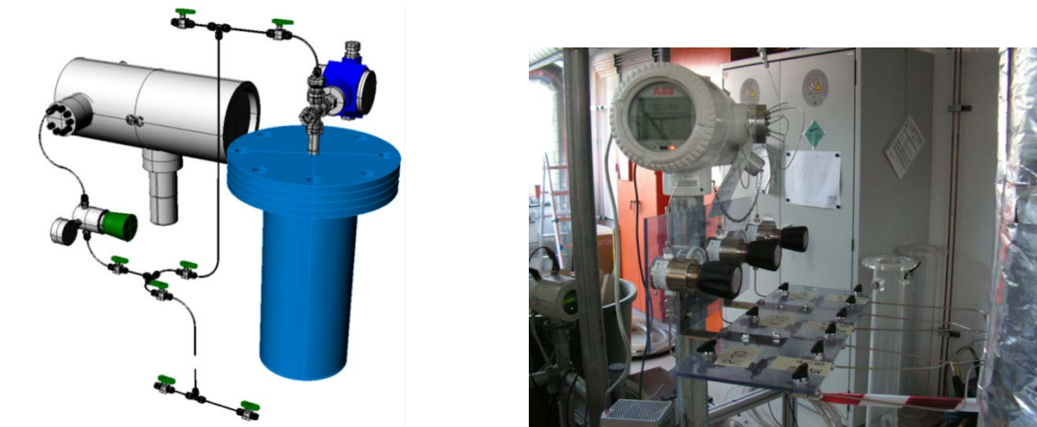
Figure 10: Process - Gas - Chromatograph with display of capillary tubes
