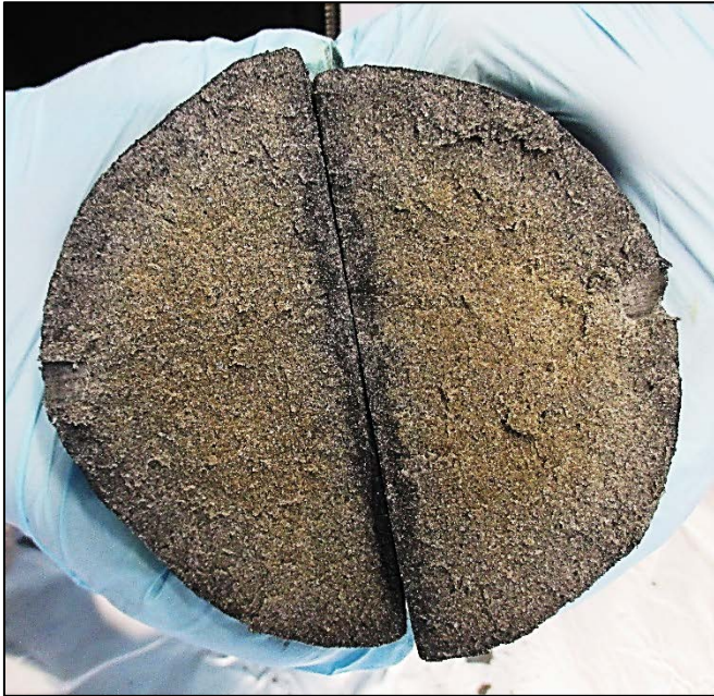
Figure 68: Discoloration of the outer edge of a drill core when the reactors are opened Source: BOKU
