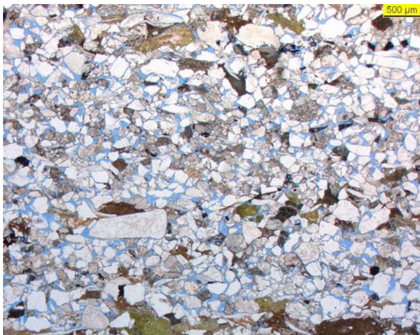
Figure 43: Overview of a porous, well sorted, fine-grained litharenite. The free pore space is blue.
