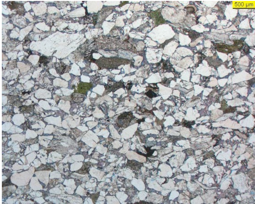
Figure 42: Moderately sorted, fine-grained, calcitically cemented litharenite
