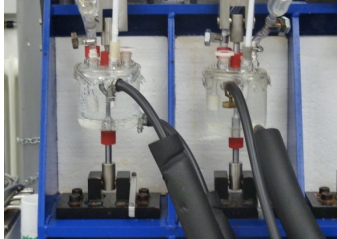
Figure 73: Test setup for CLTs at 1 bar
