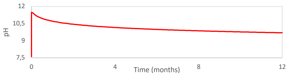
Figure 56: pH change (Basic kinetic model based on the initial system of case study 3 and assuming the reactions of pyrite and pyrrhotite are in equilibrium).
